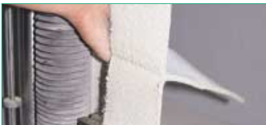
Determination of the bonded peel strength of Bentofix® geosynthetic clay liners ASTM D6496
