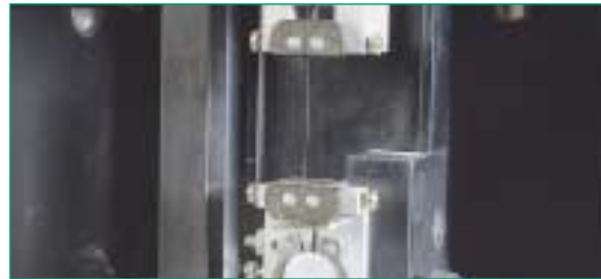
Determination of the strength and elongation properties of single fibres (DIN 53816)
