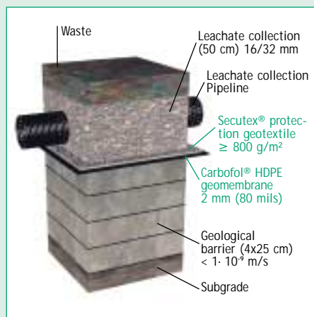
Figure 6: EU directive, state-of-practice for base seals (non hazardous)
