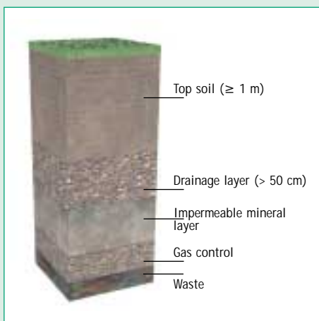
Figure 15: EU directive for landfill caps (non hazardous)
