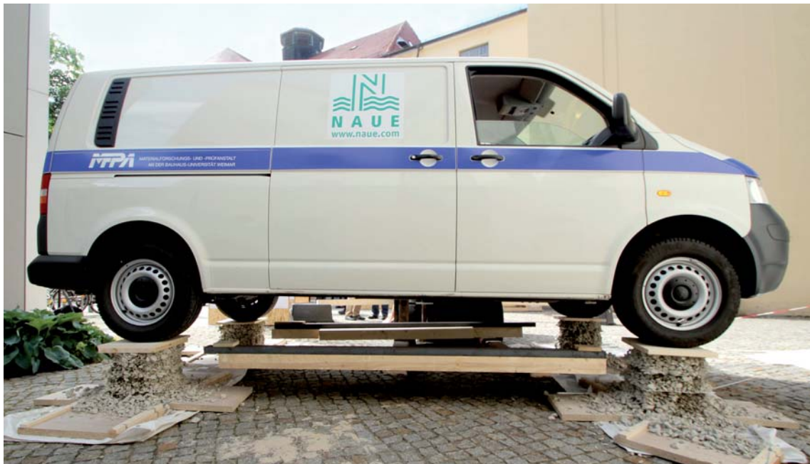
Figure 1 Shear interaction between base aggregate and Secugrid® geogrid
